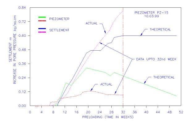
FIGURE 3.3: READINGS OF PIEZOMETER PZ-15 SHOWING CONSTANT OUTPUT
